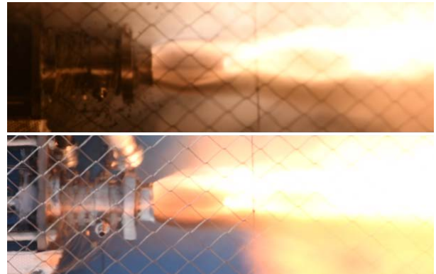
Figure 15: Liquid propellant injector HP-DSI v1.8 hot firings, with a water-cooled combustion chamber (PLD Space high pressure test bench, 2017)
