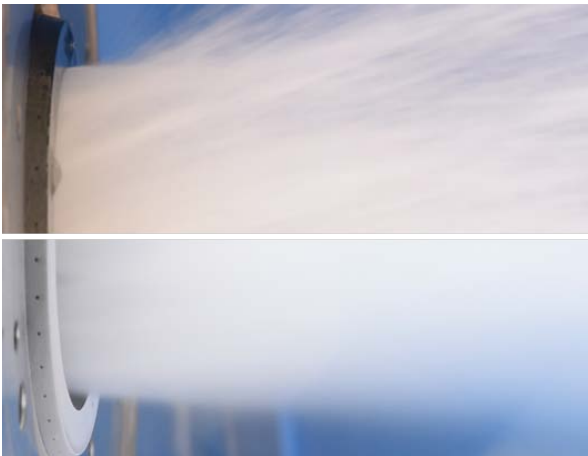
Figure 14: Cold flow test image with nominal mass flow of LOX/GN2 (bottom) and Jet A-1 (top)
