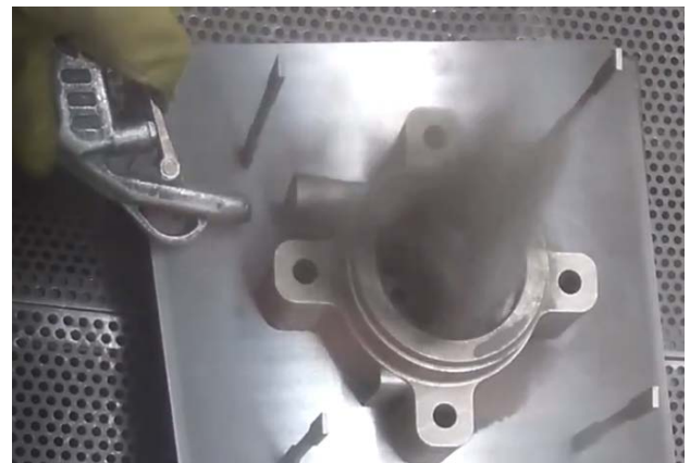
Figure 10: Illustration of the powder removal process
