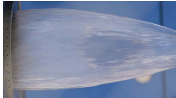
Figure 12: Pressure gradient numerical analysis of the film layer of the HP-DSI v1.8 (top) and flow test image with 90 g/s Jet A-1 (bottom)
