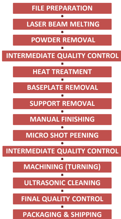
Figure 9: Manufacturing flowchart for the injector
