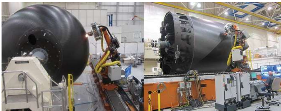
Figure 12: Carbon fibre is placed on the 5.5-meter cryotank using an automated tape placement laminator [ http://compositesmanufacturingmagazine.com/2014/10/composites-key-outer-space-applications-material/ ]
